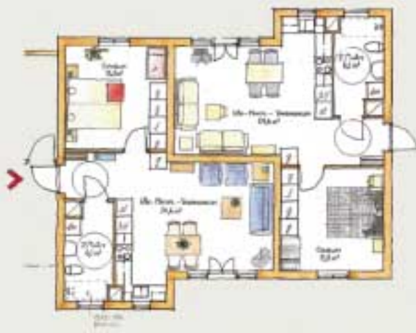
This floor plan shows space-efficient, 48-square-meter two-room apartments, equipped with bright and spacious kitchens and bathrooms with ample space for a bathtub and a washing machine. (Illustration: Origo Arkitekter AB.)
